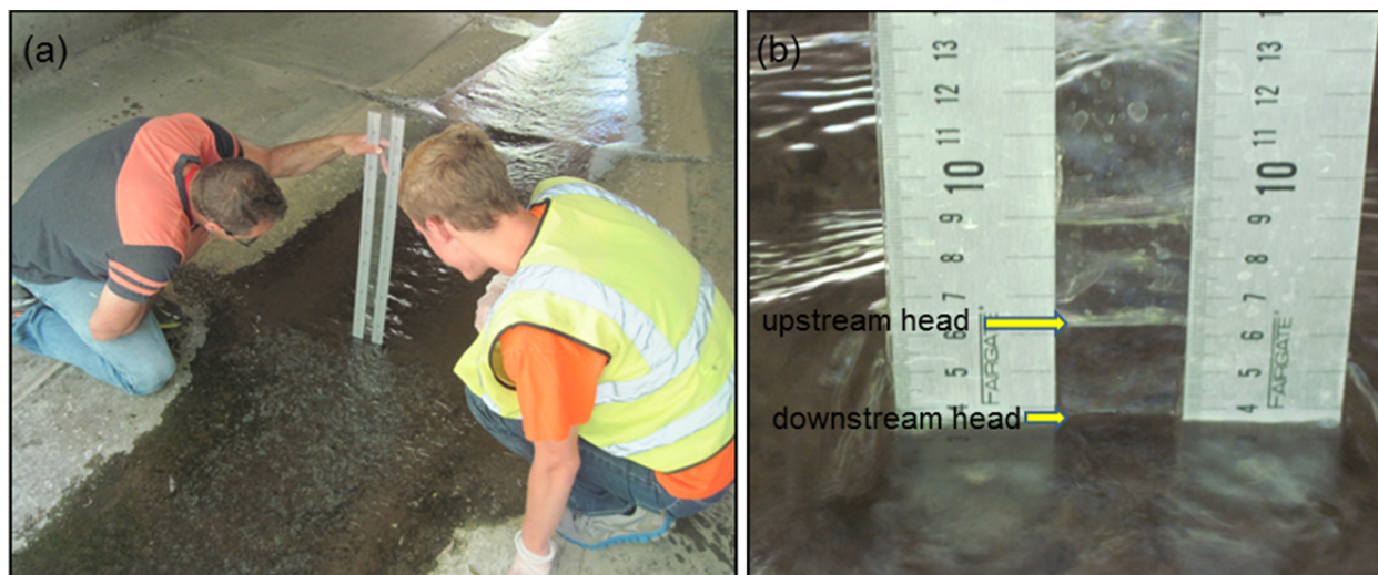
Figure 4. The use of the TVHR in Shotwell Brook at low flow: (a) TVHR in stream, and (b) difference in upstream and downstream head.
