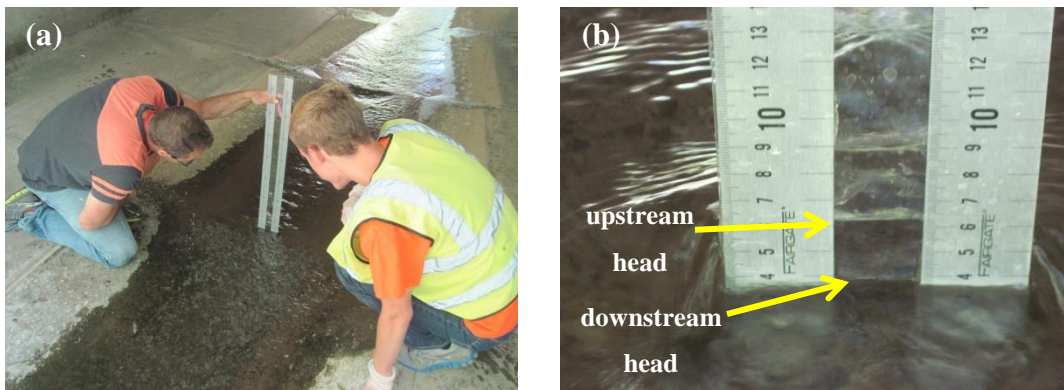
Figure 7. Measuring velocity of flow in Shotwell Brook with transparent velocity head rod (TVHR) requires the device to be held upright in stream (a). The difference in the upstream and downstream head (b) is used to calculate the velocity.
